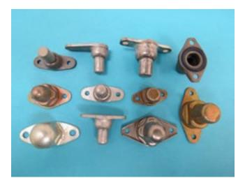
The capped styles prevent the screw threads from protruding through the nut plate. In addition, they come in a "self sealing" type which have an o-ring at the mating surface. The self sealing nut plates are available in steel and stainless steel.
